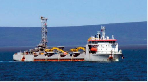
A Side Stone Dumping Vessel (SSDV) transports rocks and puts them overboard at a steady pace. This rock dumping method is typically used in shallow water.
